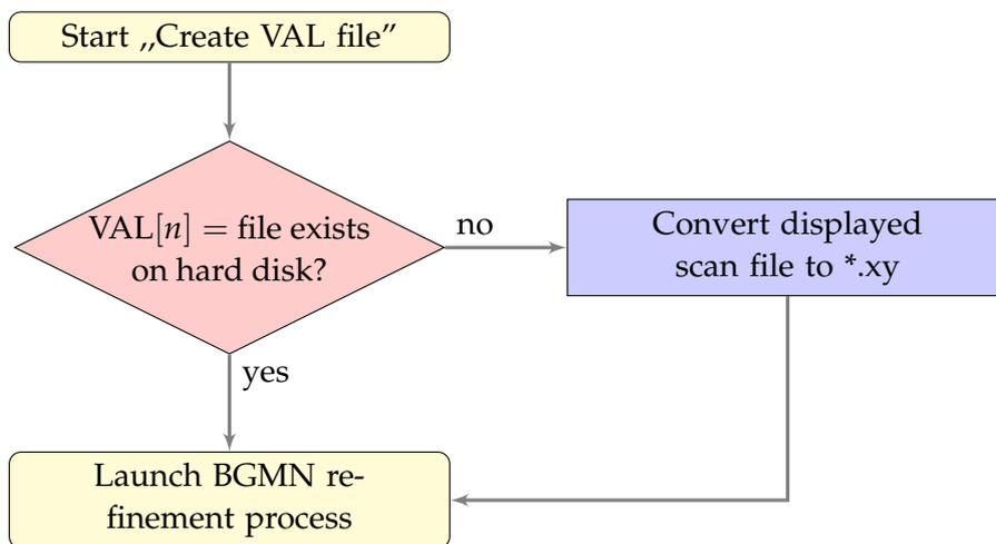
Figure 13: Immediately before running the refinement process, Profex checks whether the VAL file referenced in the control file exists on the hard disk. If not, a \*.xy file will be created from the currently displayed scan file.
