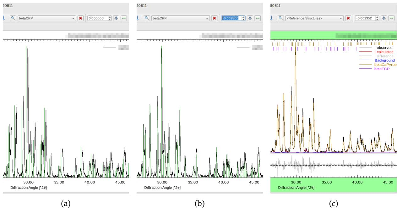
Figure 7: Sample height displacement results in a shift of the peaks in  $2\theta$ . The reference peaks no longer match the shifted measured peaks (a). Manually correcting for the shift aligns the reference peaks (b). After refinement, the refined shift is automatically applied (c).
